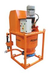
Activating colloid mixer AM 200 is designed for the preparation of high-quality cement or clay and concrete mixture in the area of special foundations construction, in rehabilitation of concrete structures, etc. The individual constituents of the mixture are activated by circulation of the dosed mixture by a centrifugal circulation pump.
